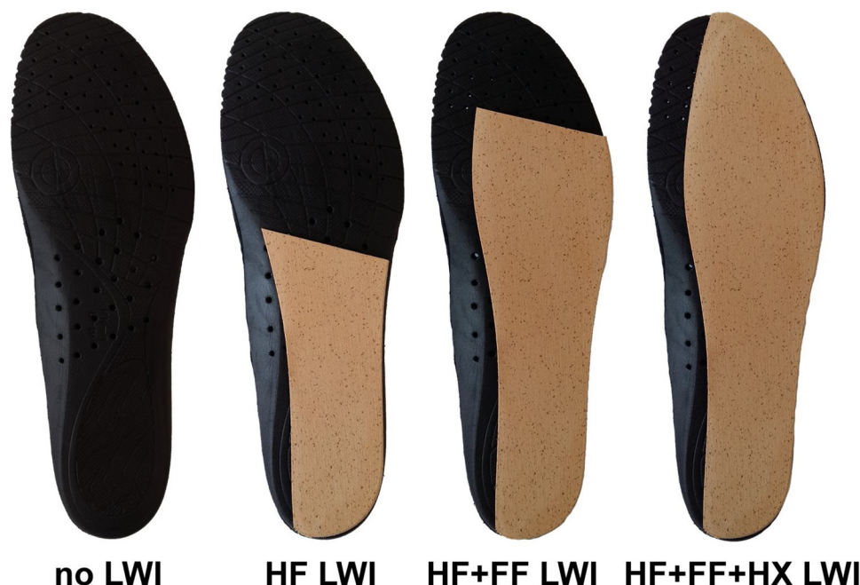
Fig. 1. Bottom view of the comfort insole with the four lengths of LWI used in this study.
