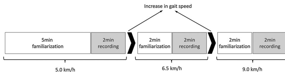
Fig. 1. Overview of a measurement session with familiarization and recording periods at each gait speed.
